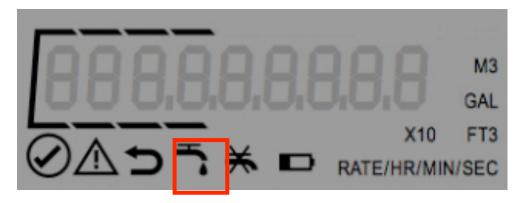
You may also identify a leak by turning off all water fixtures and water using appliances in the house and watching the meter's LCD screen to see if the odometer is increasing in value. For 5/8" to 1" meters, the odometer will show a leak as small as 0.01 gallons (GAL) per hour or 0.001 cubic feet (FT3) per hour.
